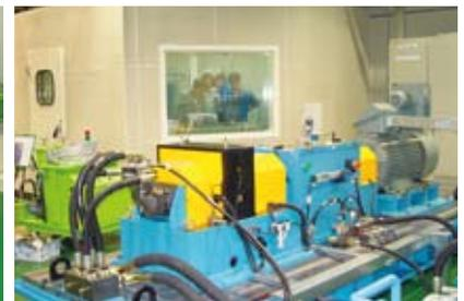
Test Object : Transmission(1200HP), Servo Cylinder, Hydro Valve, HSU (K200 & K9)
