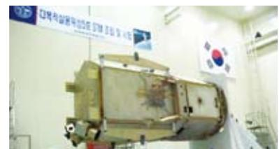
The Multi Purpose Trolley (MPT) supports the spacecraft or dedicated modules during horizontal or vertical integration and provides a table capable of tilting and rotating the spacecraft to any attitude between spin axis vertical and horizontal.
